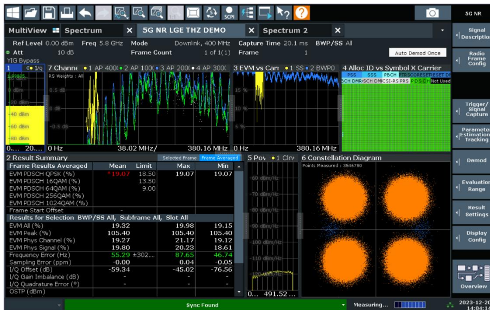
FIGURE 10 OUTPUT OF 5G NR TEST WITH VSA AND VSG
